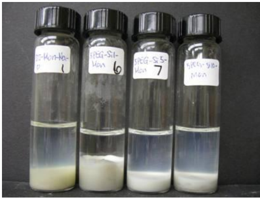
Figure 1: Picture of 10 g solution of DI water, 1, 5, and 10 wt% 5 nm PEG modified nanoparticle dispersions. Each sample contains 0.2 g clay and there is no background NaCl in the solution. The picture was taken 4 months after preparation of samples.
