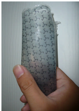
Figure 5: Flexible chiral metamaterials.
