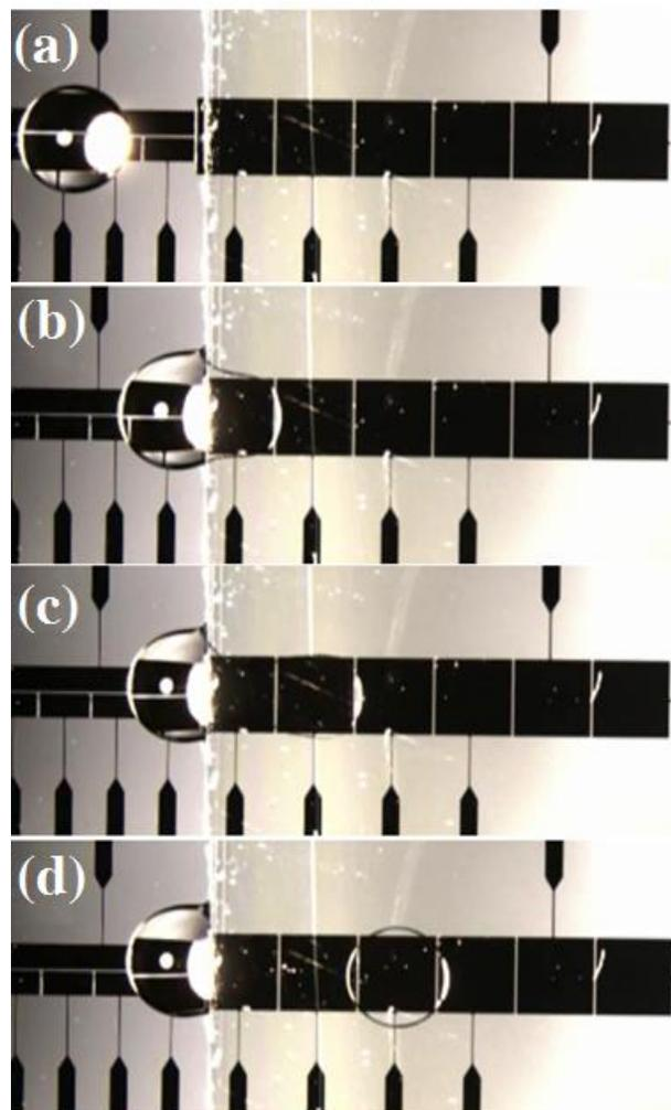
Fig. 2. Successful droplet transfer from the open to the closed DMF platform. The edge of the top plate was coated with Teflon.
