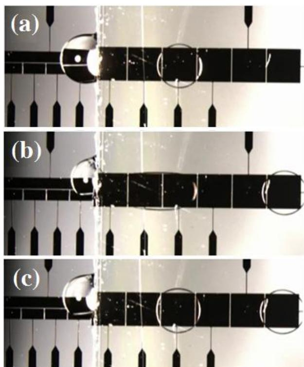
Fig. 3. Dispensing the second droplet from the same reservoir, showing the reproducibility of the dispensing process
