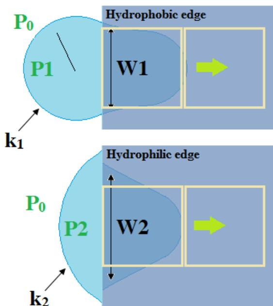
Fig. 5. Schematic of the droplet finger for both hydrophobic and hydrophilic edges of the top plate
