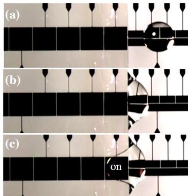
Fig. 4. Unsuccessful droplet transfer from the open to the closed DMF system. The edge of the top plate is hydrophilic
