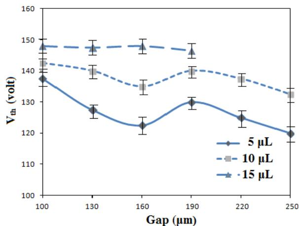
Fig. 6. Threshold voltage ( $V_{th}$ ) required for droplet dispensing based on the procedure explained in the section 3 (Experimental Procedure)
