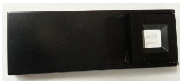
Figure 10: A cartridge for the Micro-Detectip device. The little white square on the cartridges contains the nano-size membrane on which the sensor arrays are printed
