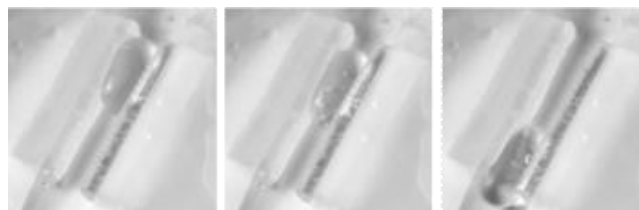
Figure 5. Demonstration of the concept for microfluidic applications (actuation and valving): (i) Initially the water plug inside the fluidic hydrophobic channel is stationary, i.e. the valve is in “closed” mode. (ii) Upon backpressure application, air pockets appear in the solid-water interface and finally (iii) the plug flows through, setting the valve in the “open” mode.
