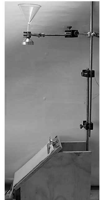
Figure 2: Impact penetration tester
