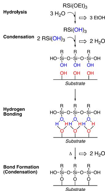
Alkoxy-silane methodology for bonding to NPs.
