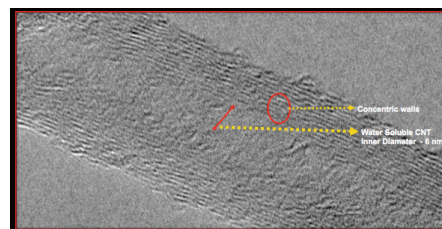
Figure 1: Multi-walled structure of water soluble Carbon Dots
