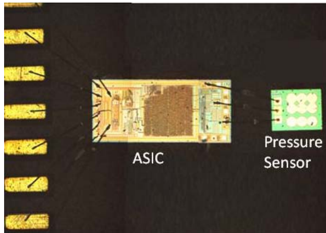
Figure 2: Microphotograph of the pressure sensor microsystem
