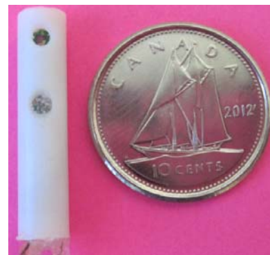
Figure 5: Packaged pressure sensor system next to Canadian 10-cent coin diameter of 18.03 mm)
