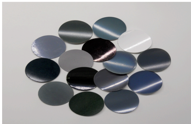
Figure 1: Various polymeric derivatives formed into membrane flatsheet coupons.
