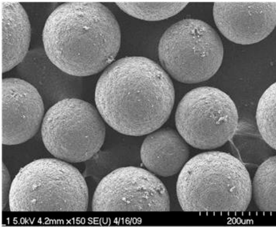
Figure 3: SEM micrograph of BrightBlack microbeads.
