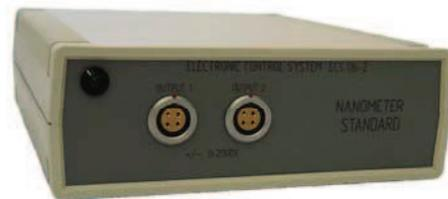
Fig.11. High voltage electronic control system.
