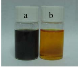
Figure 1. the optical pictures of sorted sc-SWCNTs in toluene before (a) and after (b) centrifugation.
