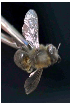
Figure 8: Copper film deposited on a bee wing using TVA.
