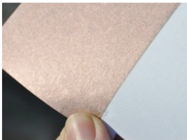
Figure 9: Paper sheet deposited with a copper film using TVA
