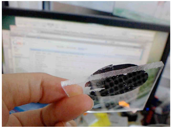
Figure 6: Diamond Like Carbon self-sustaining film (2.1 microns thickness).
