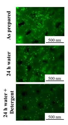
**Figure 4** Fluorescence microscope images of cotton fabric soaked for 1 hour in 0.5 weight % aqueous solutions of Polystyrene microspheres before and after exposure to pure water and water with detergent.
