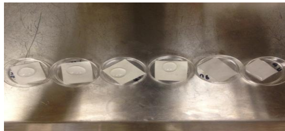
Figure1. Hydrophobicity of the HH and LH papers (first two sets respectively) compared with the untreated paper (last set).
