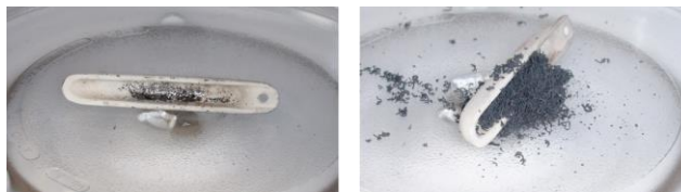
Figure 1: The expandable graphite before (left) and after (right) the microwave irradiation for 5 seconds.
