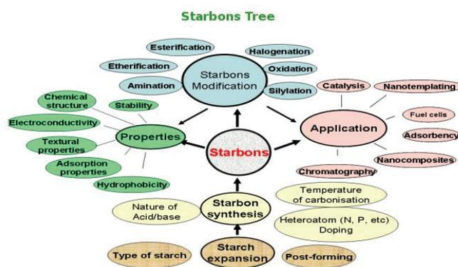
Figure 2: Starbon Tree of properties and applications
