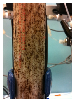
Figure 5–Picture of the glass bead pack at residual oil saturation.
