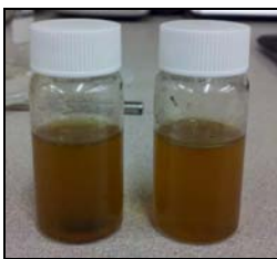
Figure 6: Upgraded bio-oil obtained from in situ hydrodeoxygenation of bio-oil during fast pyrolysis. 44% yield was obtained. The experiment was carried out using 2kg of catalyst and saw dust as the feedstock.
