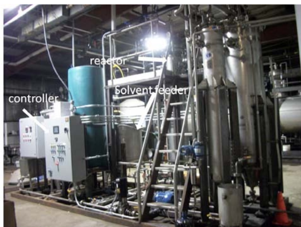
Figure 2: AST's fraction unit. This is capable of fractionating 20 kg dry biomass to produce around 4 kg of high quality lignin.
