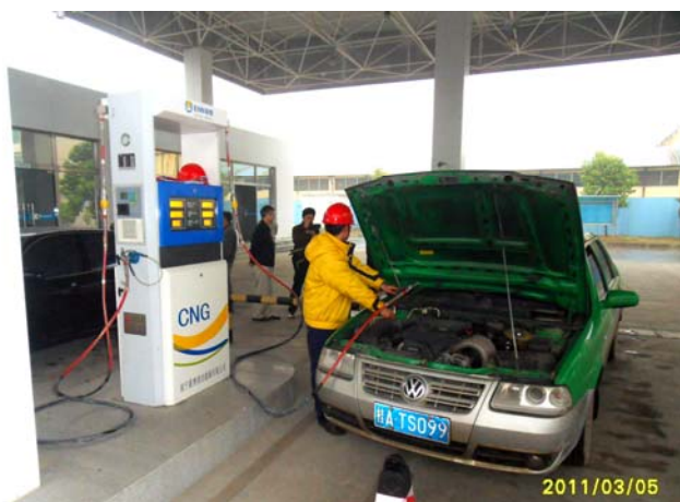
Fig 6. Methane purified from biogas is used as natural gas substitute for used as fuel by the vehicles.
