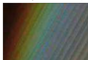
Reflected Light SiO 2 Monolayer Film 5-10 \mu m
