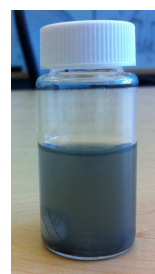
Figure 1 – Atomic layers of MoS 2 suspended in acetonitrile
