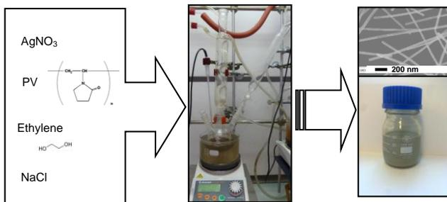
**Figure 1.** Batch synthesis of nanowires from silver salt
