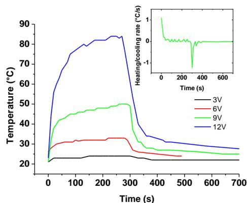
**Figure 4.** Temperature as a function of time for a  $80 \text{ ohm.sq}^{-1}$  TFH on glass at different applied voltages. Insert: derivative of the temperature vs time at 9V applied voltage.
