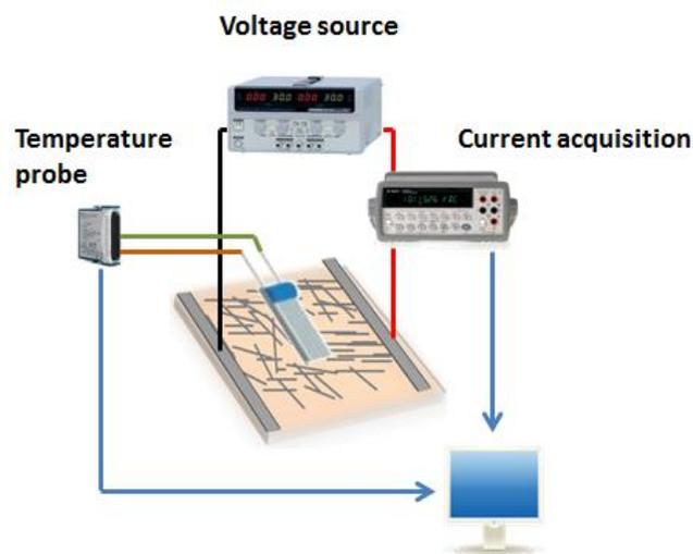
**Figure 3.** Experimental setup for monitoring heat generation of TTFHs at various voltages.
