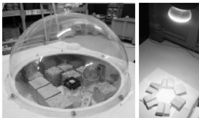
Figure 4: Carbonation chamber (left) and experimental setup for photocatalysis tests (right) on concrete specimens containing \text{TiO}_2 (model reactant: Rhodamine B dye)
