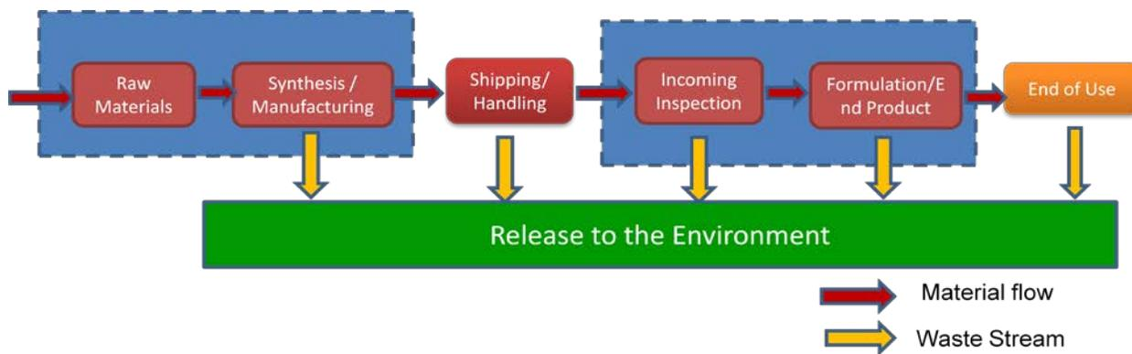
**Figure 1:** Schematic diagram depicts nanomaterial waste entering the environment from Synthesis process, the End-Product Formulation process, through product end-of-life. The Environment might be an air emission, a release into groundwater or a river, or landfill [3,5].
