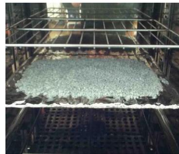
Figure 5: Baking desiccant
