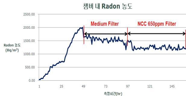
Figure 9: Filter performance test
