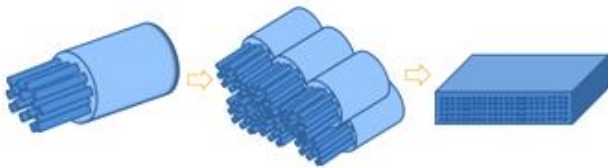
Figure 2. Fabrication process of the PAR/PET nanofiber composite by using a sheath-core fiber
