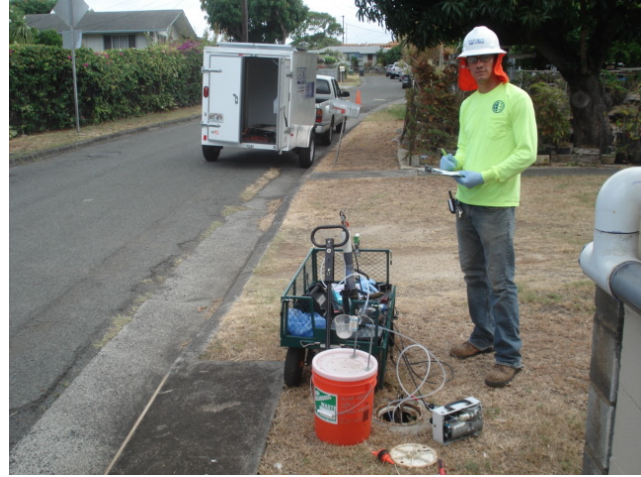
Figure 3: Battery Operated Groundwater Sampling Equipment And Solar Powered Trailer In Background
