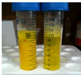
Figure 1. Left, precipitation formed with 250 μM riboflavin in water. Right, 2.0 mM riboflavin nanoemulsion.
