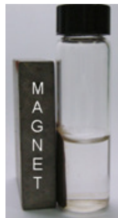
Figure 3: Separation of IO-entrapped PGMA microparticles using permanent magnet.
