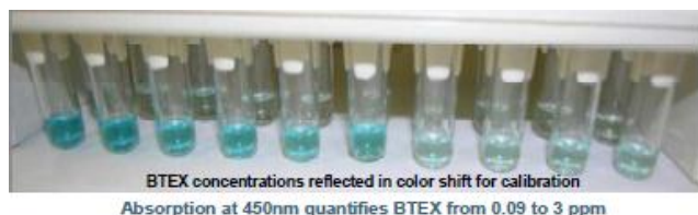
Figure 5: Calibration of ELISA assay to determine adsorption of BTEX.
