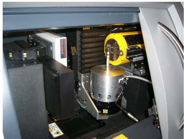
Figure 2: Thermal loading equipment installed in the computer tomography system “Nanotom”
