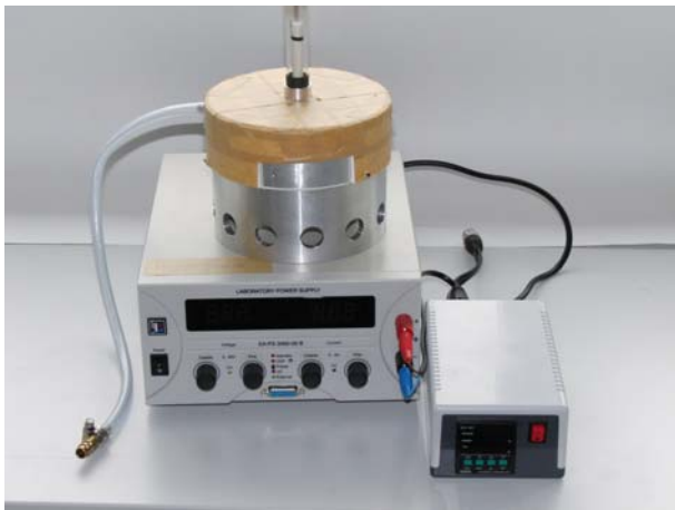
Figure 1: Thermal loading equipment for the computer tomography with power supply and temperature controller
