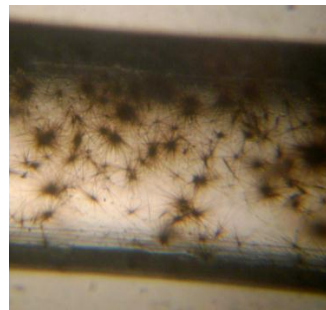
Fig 4: Optical micrograph of NWs inside microchannel.
