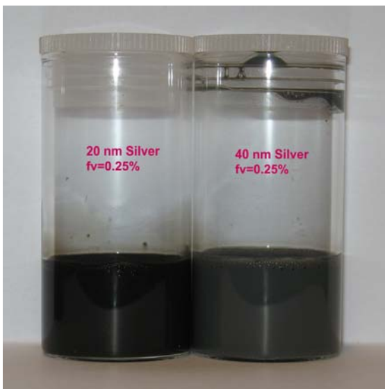
Figure 1: Silver nanoparticles dispersed in water and SDS surfactant solution
