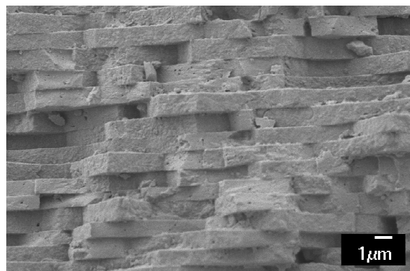
Figure 1: SEM image of the cross-section of a common mussel shell.
