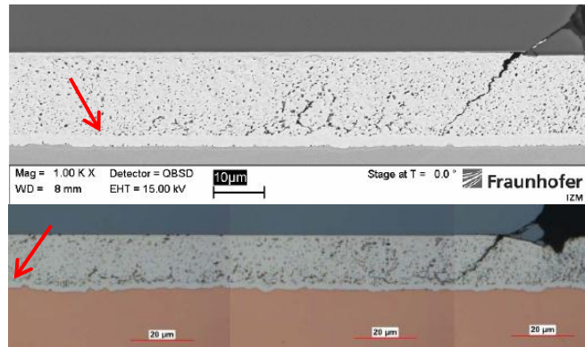
Fig. 11: Crack propagation in die attach after 1000 TC (top) and after 2000 TC (bottom) @ -55°C/125°C. The red arrow pinpoints the tip of the crack.
