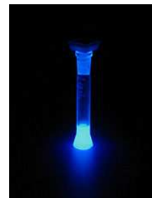
Fig.2. Chemiluminescence of luminal molecules in presence of hydrogen peroxide ( H_2O_2 )
