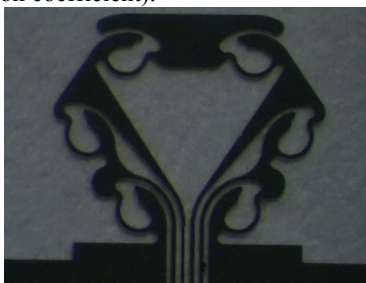
Figure 8: silicon prototype with 4 actuating cables.
