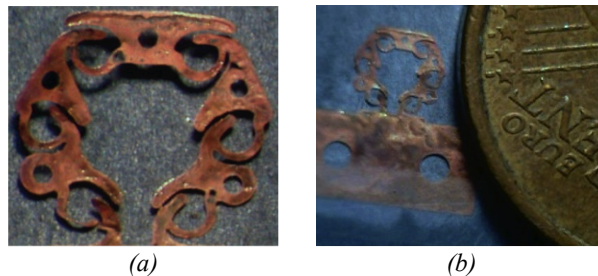
Figure 5: One sample of copper prototypes a) and a comparison of it to a 1 Euro cent coin b).
