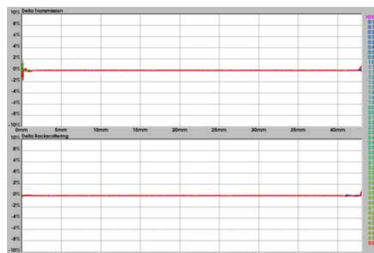
Figure 2. Transmission (top) and backscattering (bottom) for formulation 1 at 25°C
