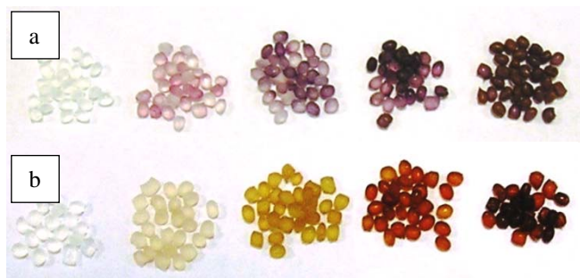
Figure 1: (a) nanogold-polyurethane and (b) nanosilver-polyurethane hybrids; the shade and intensity of the colour increase with increasing nanogold and nanosilver content respectively.
