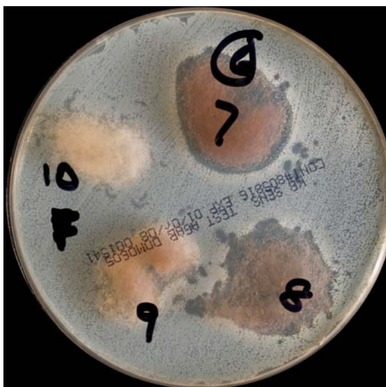
Figure 6: Inhibition zones of Staphylococcus aureus microbial growth by merino wool - silver chloride nanoparticle composites loaded with (7) 4.9 wt % Ag; (8) 3.8 wt % Ag; (9) 2.2 wt % Ag; (10) 1.3 wt % Ag.
