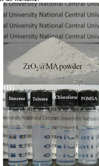
Figure 1: The MA modified ZrO 2 nanoparticles in dried powder form and its 10 wt% dispersion in selected solvents.
