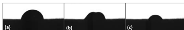
Figure 4. Images of the sequence of oil separation from a drop of oil/water mixture.
