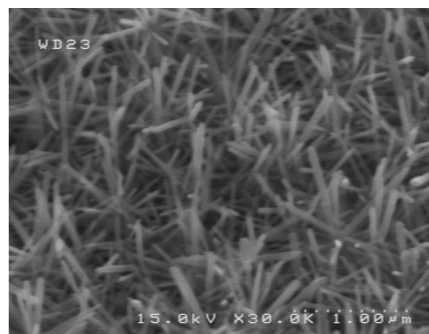
Fig. 4: SEM images of the growth ZnO NR -MWCNT heteronanostructure under different growth temperature: (a) 60°C, (b) 80°C, (c) 95°C and The precursor concentration and and time were 12mM and 4 h, respectively.
