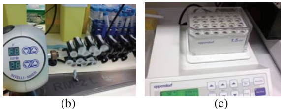
Figure 2. (a) Binding efficiency of DNA on silica beads for rotary mixer and Thermomixer; (b) Rotary Mixer; (c) Thermomixer.
