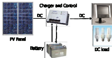
Figure 3: PV stand-alone system supply to DC load (with charger and controller)
