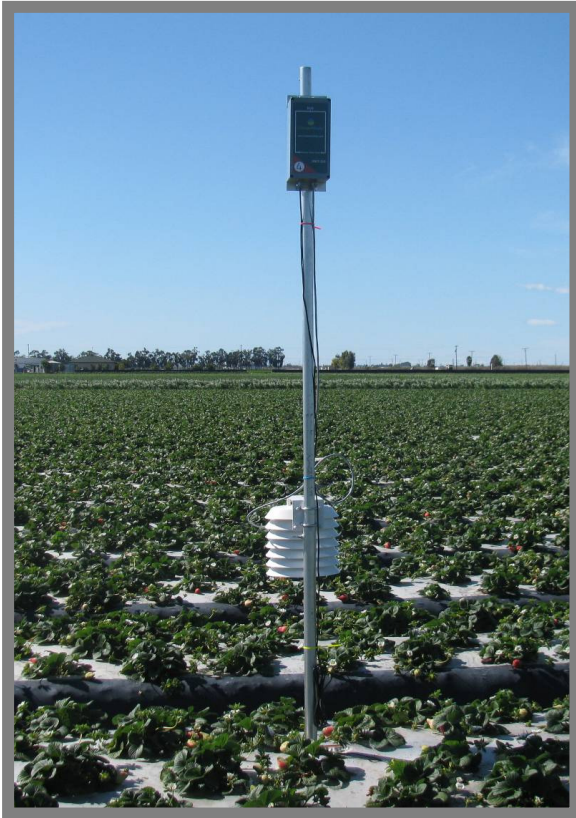
Figure 5: ClimateMinder Wireless Sensor Node in a Strawberry Field
