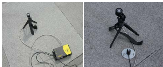
Figure 6: The whole set of the spectroradiometer and comparison with the pyranometer on the right.
