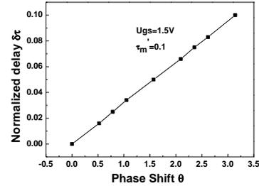
Fig.4 The delay as a function of phase shift  $\theta$ , the value of the friction parameter is  $\gamma = 2.02$ . The gate-to-channel voltage is  $U_g = 1.5 \text{ V}$ , the source and drain ac amplitudes are  $u_a = u_b = 0.01 \text{ V}$ , ac frequencies are given by  $f_a = 1.07 \text{ THz}$  and  $f_b = 3.21 \text{ THz}$ .
