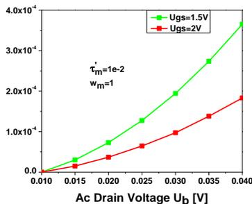
Fig.8 Induced dc component of the source current density as a function of the ac amplitude of the applied drain voltage in the case of equal frequencies of the source and drain potentials. The green line is simulated by  $U_{gs} = 1.5V$  and the red curve is simulated by  $U_{gs} = 2V$ . Some parameters used here are  $\tau_m = 0.01, w_m = 1$ .
