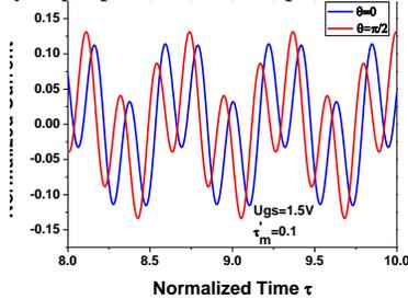
Fig.3 Source current density as a function of time. The value of the friction parameter is  $\gamma = 2.02$ . The gate-to-channel voltage is  $U_g = 1.5 \text{ V}$ , the ac amplitudes of signals at the source and drain are  $u_a = u_b = 0.01 \text{ V}$ , ac frequencies are given by  $f_a = 1.07 \text{ THz}$  and  $f_b = 3.21 \text{ THz}$ . The solid curve is obtained from the numerical solution of the nonlinear equations.
