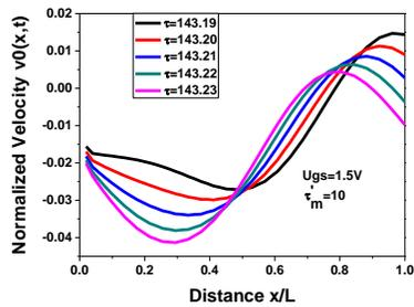
Fig.7 (b).Velocity at different time as a function of  $x/L$ , where  $L$  is channel length. The values of normalized time are 148.25, 148.26, 148.27, 148.28, and 148.29. Some parameters used here are  $\tau_m = 10, f_a = 1.07THz, f_b = 3.021THz$
