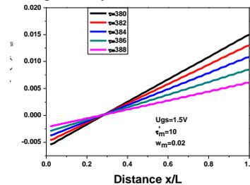
Fig.6 Electron density variation corresponding to the case of  $\gamma = 0.0202$ ,  $f_a = 13.49 \text{ GHz}$  and  $f_b = 40.47 \text{ GHz}$ .
