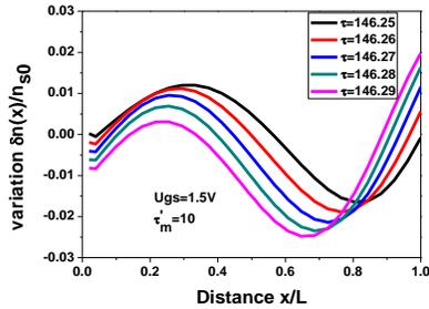
Fig.7 (a).The electron density variation is plotted at different times as a function of  $x/L$ , where  $L$  is channel length. The values of the normalized time are 148.25, 148.26, 148.27, 148.28, and 148.29. Parameters used in the simulation are  $\tau_m = 10, f_a = 1.07THz, f_b = 3.021THz$
