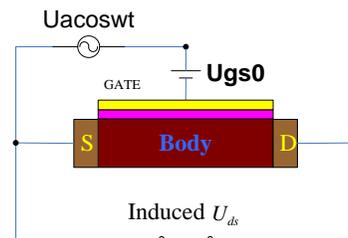
Fig.1 The equivalent circuit for terahertz detection induced by radiations between source-and-gate electrodes of device
