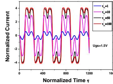
Fig.5 Source current density as a function of time with different friction parameters  $\gamma : 0.202, 0.0202, 0.00405, 0.00202$ . The gate voltage swing is  $U_g = 1.5 \text{ V}$ , the source and drain ac amplitudes are  $u_a = u_b = 0.01 \text{ V}$ , ac frequencies are given by  $f_a = 13.49 \text{ GHz}$  and  $f_b = 40.47 \text{ GHz}$ .
