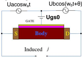
Fig.2 Equivalent circuit for measuring response of FET device to harmonic signals applied at source and drain sides
